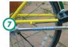
Unique Shaft drive instead of the chain
