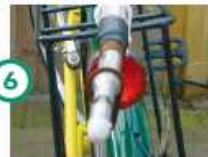
Stainless steel locking cord attached to the bike with a microchip at the end which inserts into the rental station
